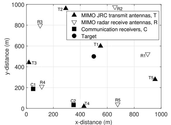
Fig. 4: Simulation layout for distributed JRC MIMO system.
