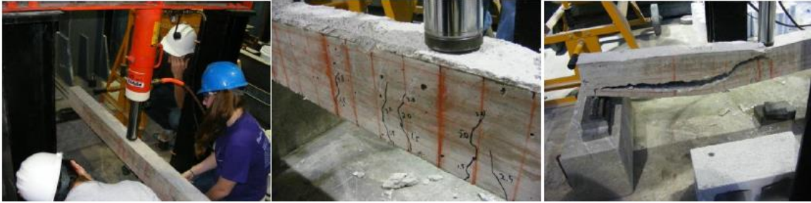
Figure 5. Crack mapping of reinforced concrete beams.
