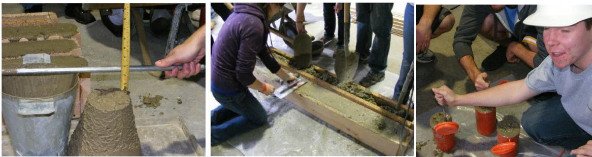
Figure 3. Slump testing and pouring of concrete beams and cylinders.
