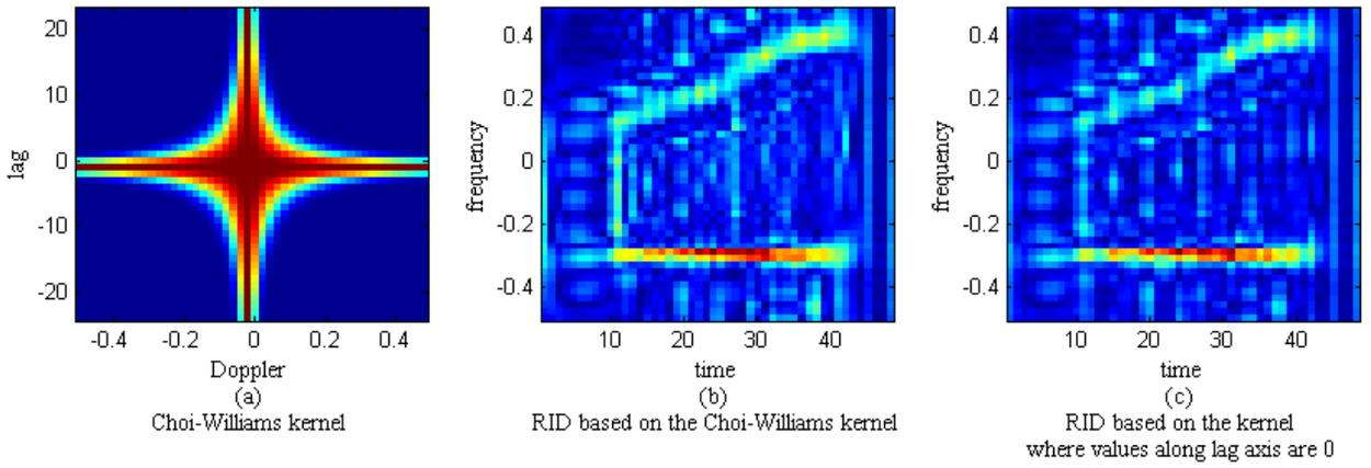
Figure 3. Reducing the effect of impulses by imposing the zero values along the lag axis in the ambiguity domain.
