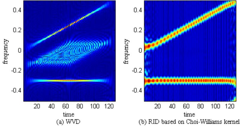
Figure 2. TFRs of a signal consisting of a sinusoid and a chirp.
