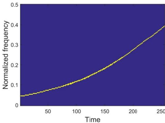
Fig. 3. Sparse reconstruction using chirp dictionary
