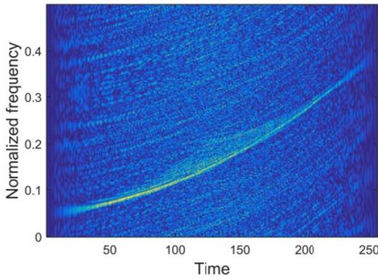
Fig. 2. WVD of the jammed GPS signal
