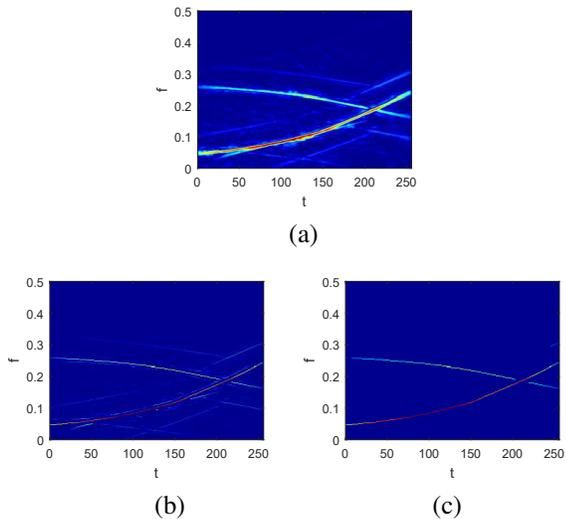
**Fig. 4** The TFRs obtained by applying the proposed techniques to the received signal of Fig. 2(a): (a) ADTFD with SPWVD as the underlying TFD; (b) Resulting TFR after smoothing the TFR of Fig. 4(a) using global thresholding; (c) Proposed ALF-DTFD ( $M=1$ ,  $Q=256$ ,  $\xi=0.41$ ).
