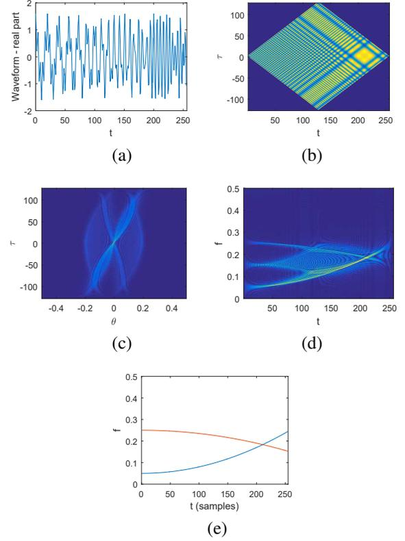
**Fig. 1** The original signal without missing samples: (a) Real part of the signal; (b) IAF; (c) AF; (d) WVD; (e) True IFs.
