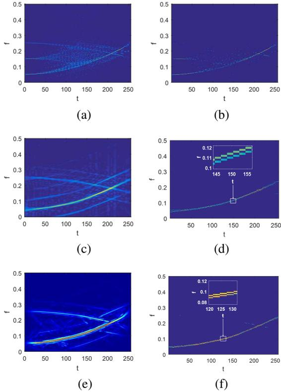
**Fig. 3** The TFRs obtained using different existing approaches applied to the received signal of Fig. 2(a): (a) MIAA applied to the IAF; (b) OMP applied after MIAA; (c) AOK; (d) OMP applied to the kered IAF obtained from the AOK; (e) ADTFD with WVD as the underlying TFD; (f) OMP applied after the ADTFD.
