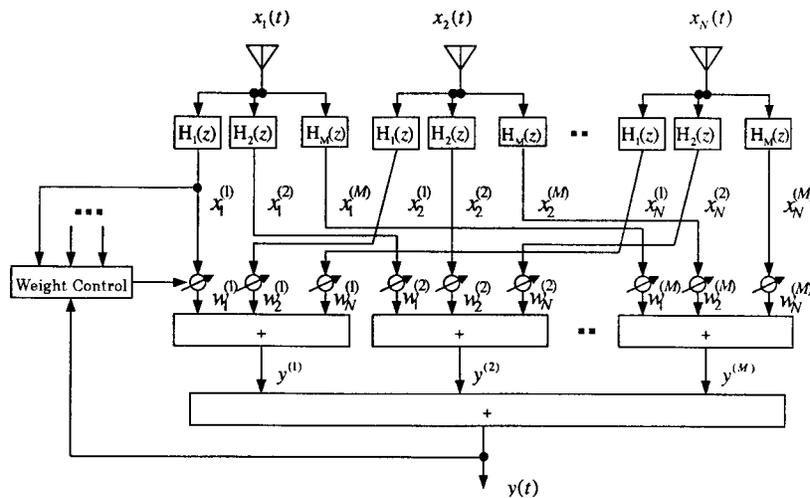
Fig. 4. A subband CMA adaptive array.
