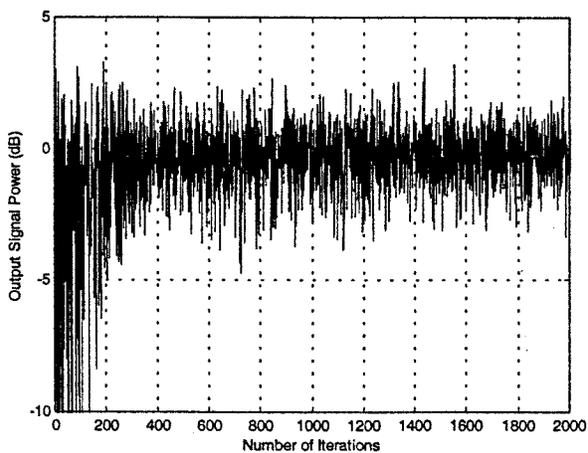
(c) Output signal power of the array (with subband processing :  $M=8$ )
