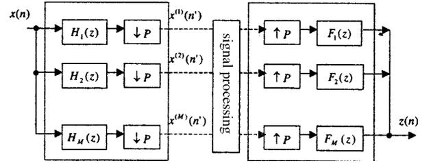
Fig. 2. Subband signal processing by filter banks.
