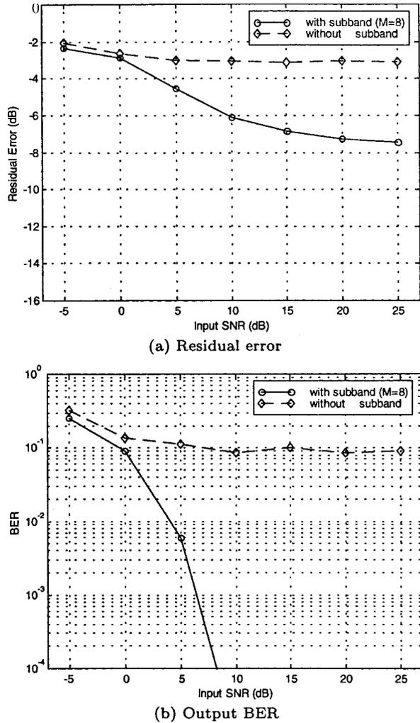
Fig. 8. The array performance when the number of rays exceeds array DOFs ( $N = 3$ ,  $\sigma_{D1}^2 = 0$  dB,  $\sigma_{D2}^2 = -3$  dB,  $\phi_{D1} = 0^\circ$ ,  $\phi_{D2} = 20^\circ$ ,  $\tau_D = T_S$ ,  $\sigma_{I1}^2 = -3$  dB,  $\sigma_{I2}^2 = -6$  dB,  $\phi_{I1} = -20^\circ$ ,  $\phi_{I2} = -60^\circ$ ,  $\tau_I = T_S$ ,  $\sigma_n^2 = -10$  dB).
