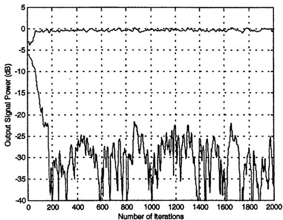
(b) Output signal power of the two rays (without subband processing)
