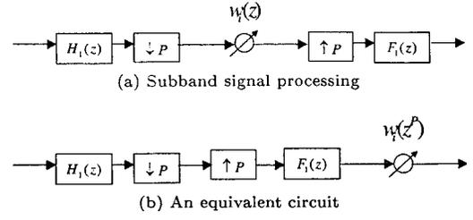
Fig. 3. Subband signal processing and its equivalent circuit.
