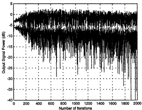
(d) Output signal power of the two rays (with subband processing :  $M=8$ )
