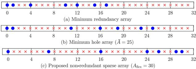
Fig. 1. Sensor positions for sparse arrays being compared ( $N = 7$  sensors).
