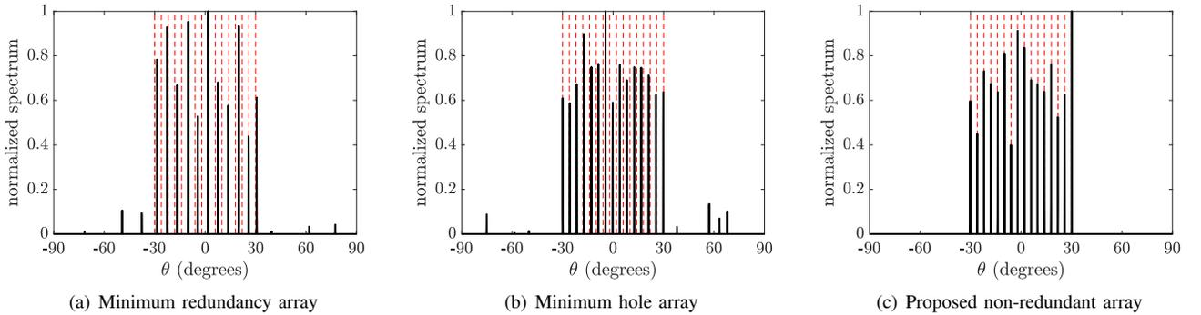
Fig. 4. LASSO spectra for  $Q = 16$  sources uniformly distributed from  $-30^\circ$  to  $30^\circ$  using the sparse arrays consisting of  $N = 7$  sensors ( $M = 500$  snapshots,  $\text{SNR} = 0$  dB,  $\bar{A} = 25$ ,  $A_{\text{flex}} = 30$ ).
