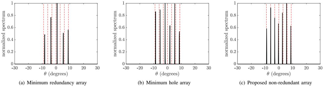
Fig. 3. LASSO spectra for  $Q = 7$  sources uniformly distributed from  $-9^\circ$  to  $9^\circ$  using the sparse arrays consisting of  $N = 7$  sensors ( $M = 500$  snapshots,  $\text{SNR} = 0$  dB,  $\bar{A} = 25$ ,  $A_{\text{flex}} = 30$ ).
