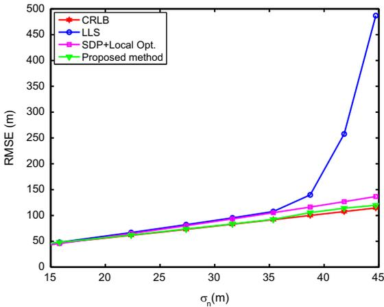
Fig. 4. RMSE performance versus noise variance with uniformly distributed receiver position error  $d = 12$  m.
